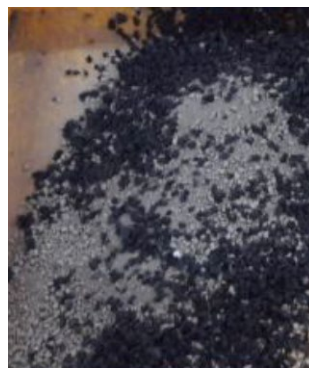
Fig. 3 - The mixture of recycled waste tyre granules and clay soil
