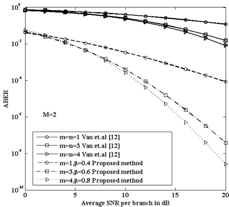
Fig. 7 – Comparison of ABER vs average SNR between the proposed system over  $K_G$  fading channel and that given in Van et.al [12] for Nakagami fading channel
