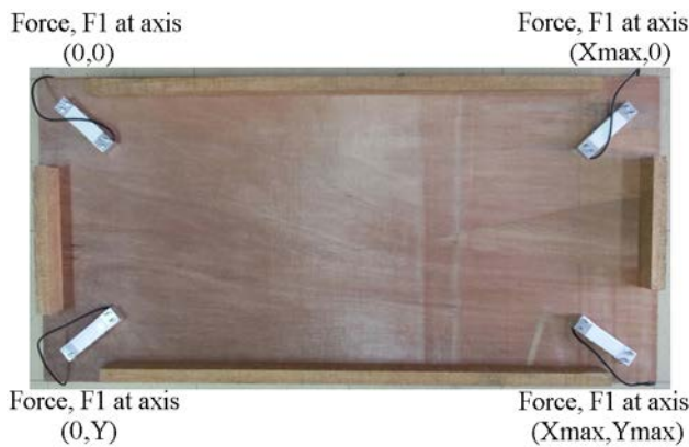
Fig. 4 Load cell placements
