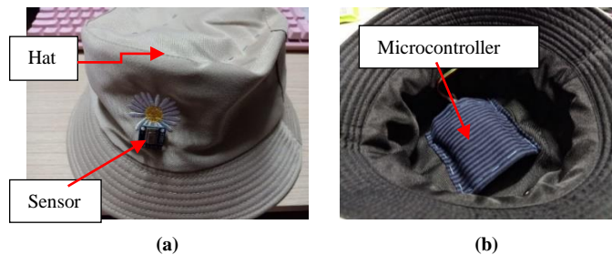
Fig. 4 - (a) Front view and; (b) bottom view of the wearable non-contact temperature detector
