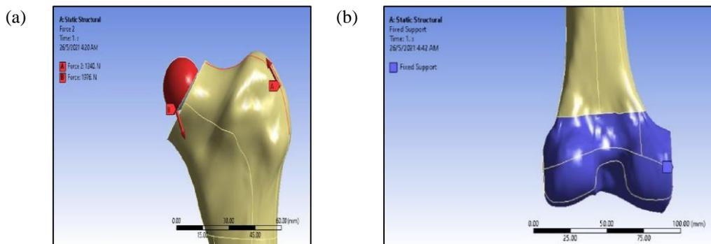
**Fig. 5 - The location of (a) the force exerted; (b) fixed support on the distal end of the bone**
