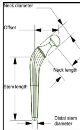
**Fig. 3 - Hip implant parts labelling**
