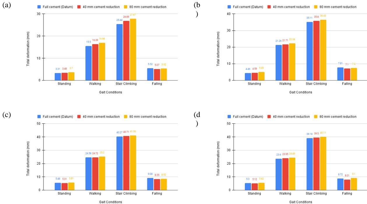
**Fig. 6 - Graphs of total deformation for cements with Young Modulus of (a) 2.24 GPa; (b) 0.3129 GPa; (c) 0.03394 GPa; (d) 0.07961 GPa**
