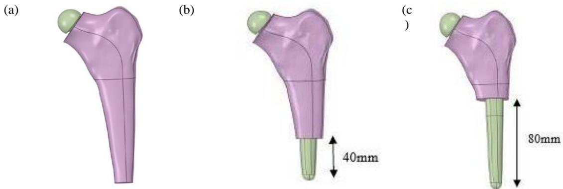
**Fig. 4 - The types of proximal cementation used in this study (a) fully cemented; (b) 40 mm cut off; (c) 80 mm cut off [26]**
