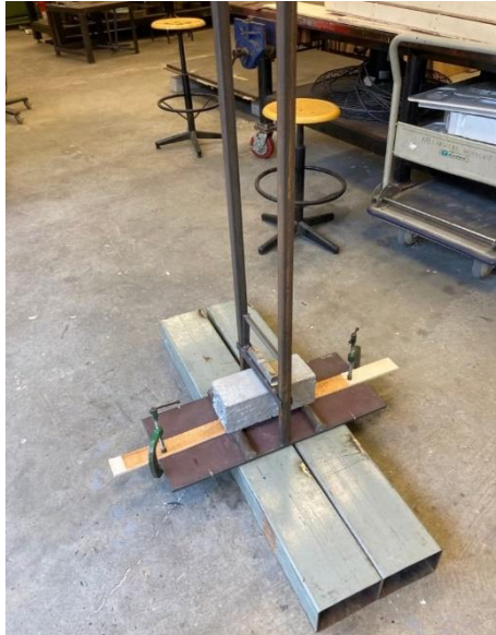
Fig. 3 - Experimental setup of repeated impact drop weight test (200 mm span)
