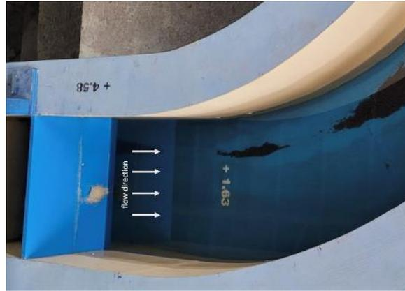
**Fig. 15 - Accumulated sediment remaining at the downstream channel with the modified design**
