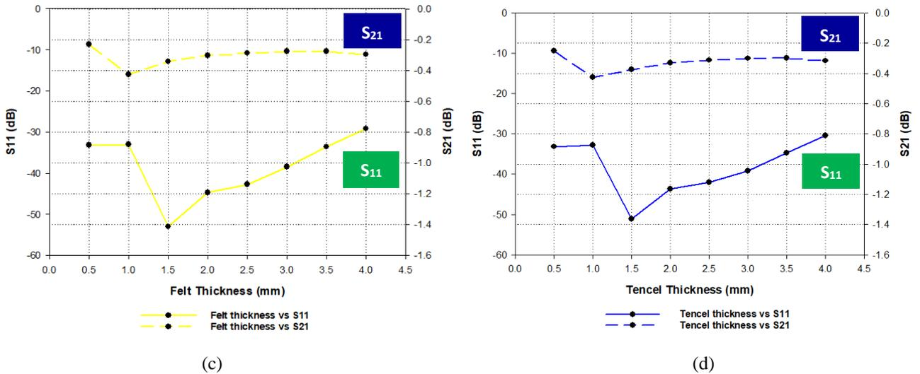
Fig. 5 - S<sub>11</sub> and S<sub>21</sub> performance plots for fabric of (a) Rogers 5880, (b) denim, (c) felt and (d) Tencel
