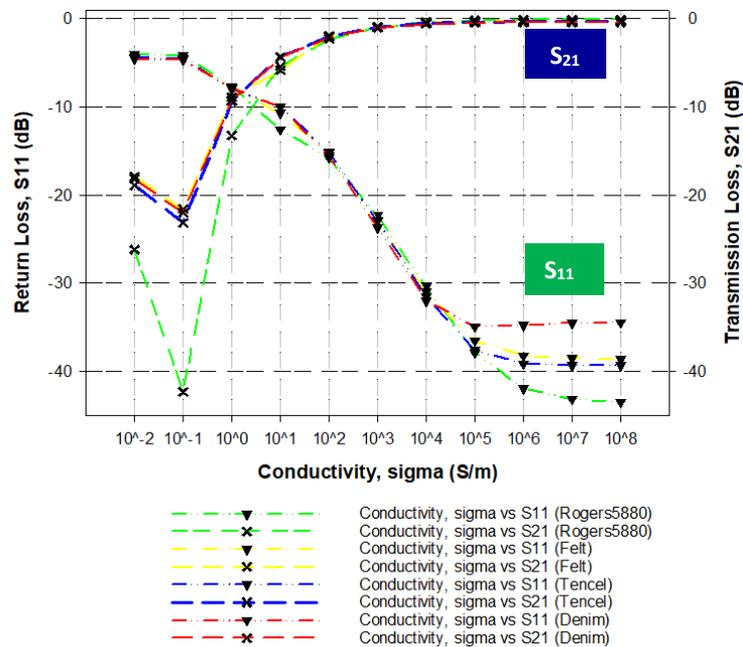
Fig. 7 -  $S_{11}$  and  $S_{21}$  versus conductivity plot
