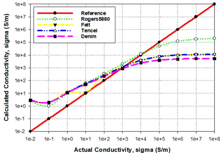
Fig. 9 - Actual and calculated values of conductivity of Rogers 5880, felt, Tencel and denim
