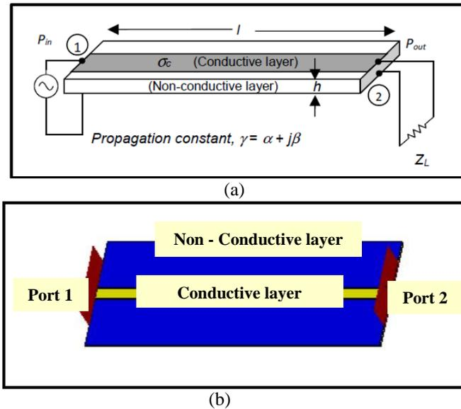
**Fig. 3 - (a) Two-port transmission line model (b) Two-port transmission line model design in CST**
