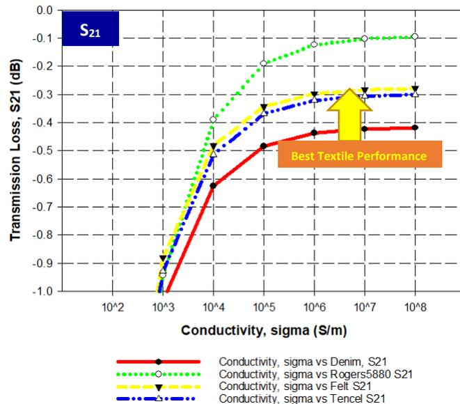
Fig. 8 - Refinement plot of  $S_{21}$  versus conductivity plot
