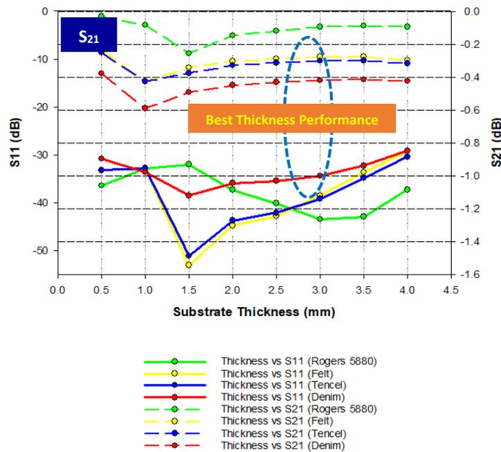
Fig. 6 - Merged plot of S<sub>11</sub> and S<sub>21</sub> performance for denim, felt, Tencel and Rogers 5880
