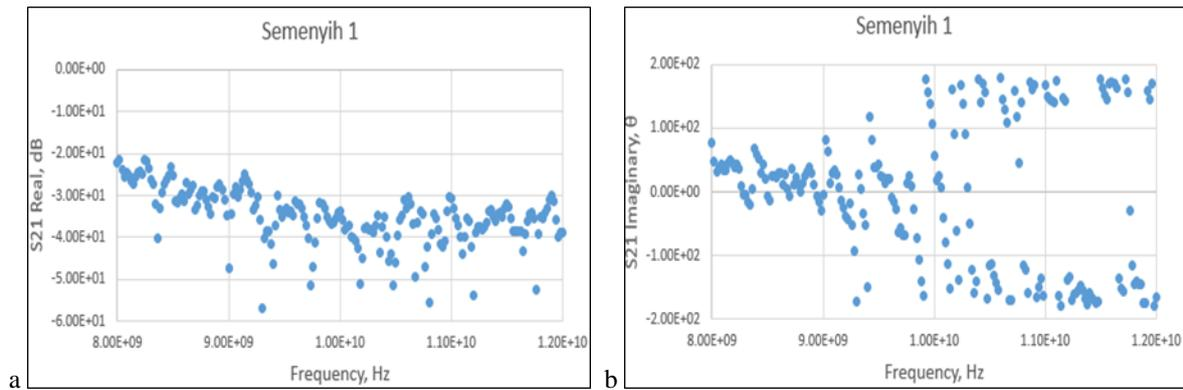
**Fig. 5 - Scattering plot of  $S_{11}$  against frequency for sample 1 from Semenyih 2 plant (a)  $S_{21}$  real; (b)  $S_{21}$  imaginary**
