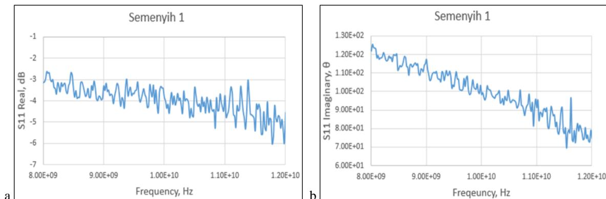
Fig. 2 - Graph of  $S_{11}$  against frequency for sample 1 from Semenyih 2 plant (a)  $S_{11}$  real; (b)  $S_{11}$  imaginary
