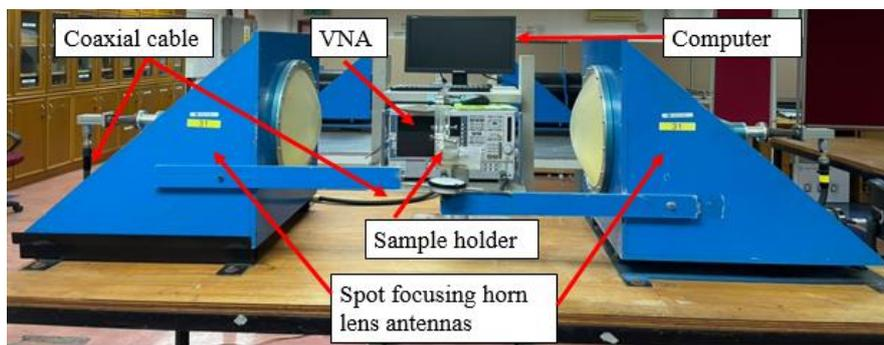
**Fig. 1 - MNDT (free space) measurement setup**
