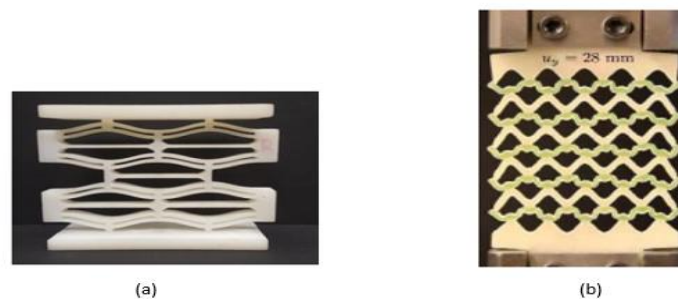
Fig. 3 - (a) Negative stiffness honeycomb structure [10] and; (b) different meta-material honeycomb structure under tension [11]
