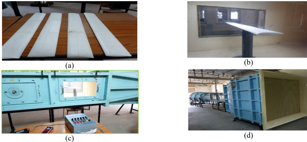
Fig. 3 - Wind tunnel set-up (a) 3D-printed models; (b) strain guage balance platform; (c) 6-D component system; (d) LSWT
