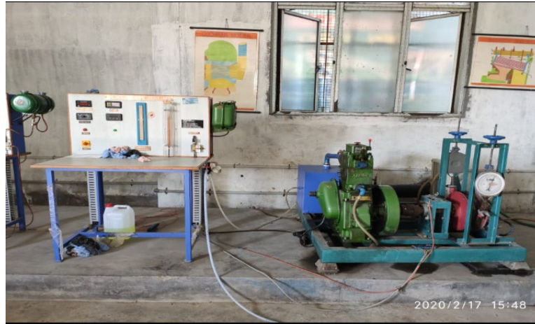
Fig. 1 - View of the experimental setup with a four-stroke CI diesel engine
