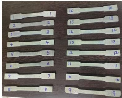
Fig. 15 - Before tensile test 16 samples
