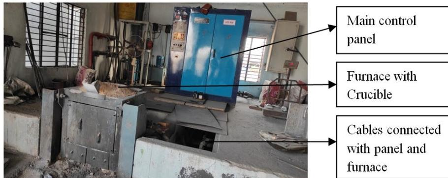
**Fig. 1 - Medium frequency induction furnace**
