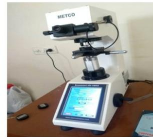
Fig. 11 - Vickers Micro hardness machine
