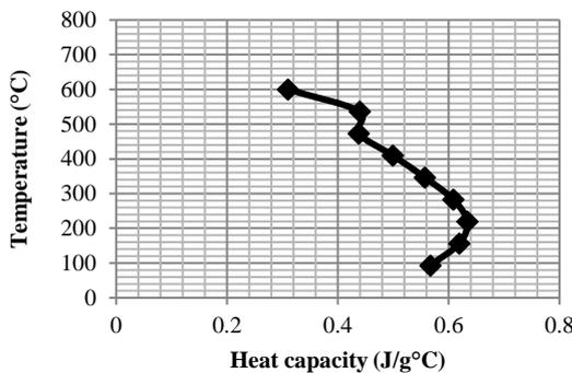
Fig. 2 Specific heat capacity of Aloji fireclay
