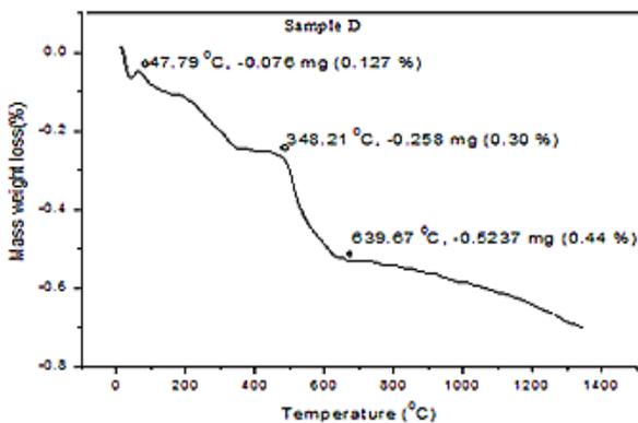
Fig. 4 TGA curve for Aloji fireclay brick
