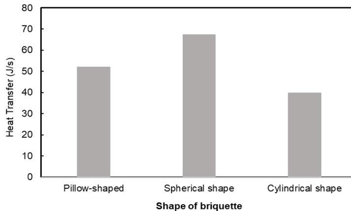
Fig. 4 Heat transfer rate of each briquette shapes
