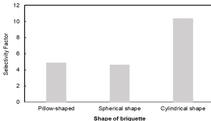
Fig. 8 Selectivity factor value from each briquette shapes
