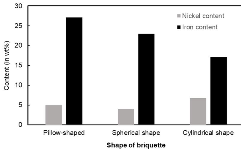
Fig. 5 Nickel and iron content of each briquette shapes
