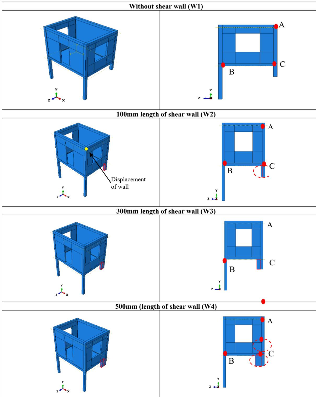
Fig. 11 - Different shear wall lengths at the short column
