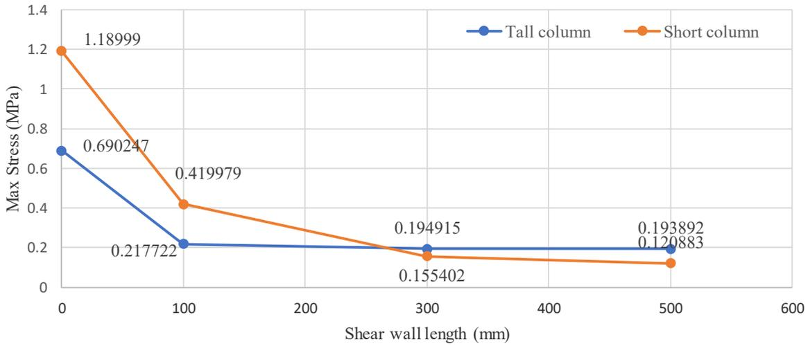
Fig. 14 - Maximum stress at tall column and short column
