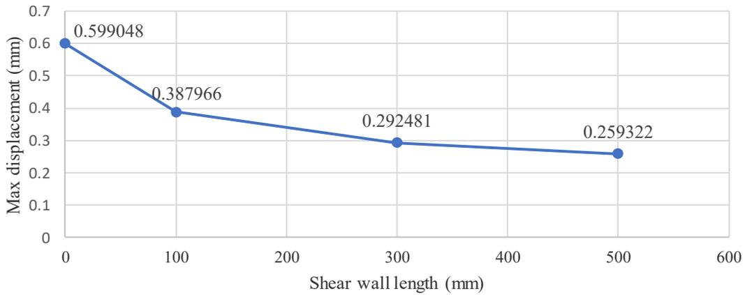
Fig. 12 - Maximum displacement of frame with different shear wall length
