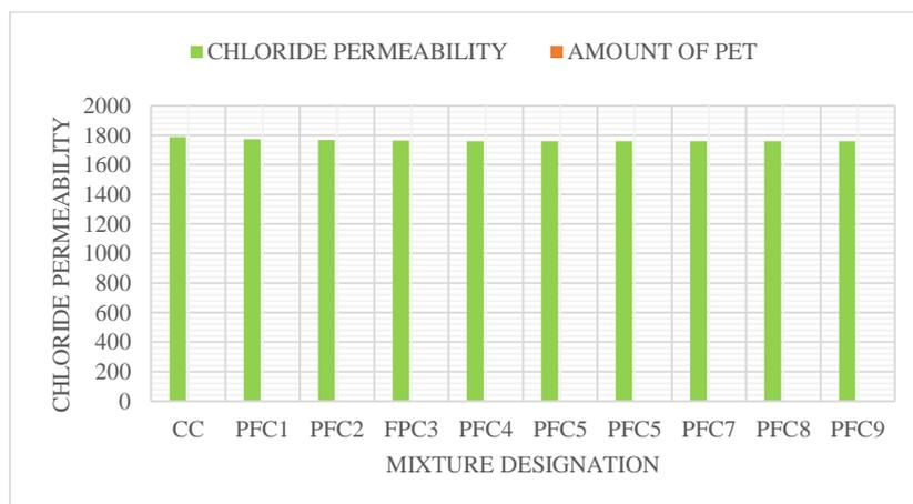
**Fig. 5 - Chloride permeability reading for the sample mixes with plastic [59]**
