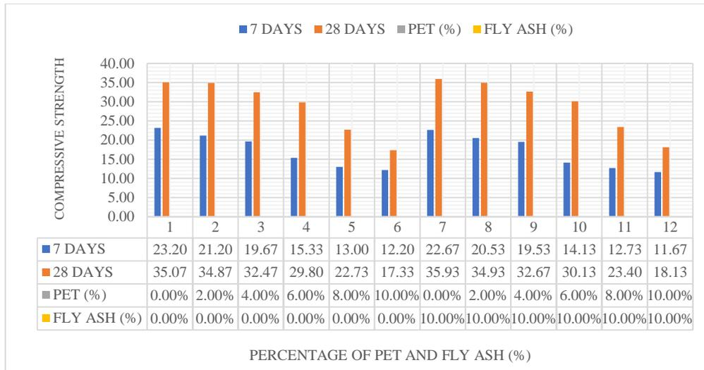
Fig. 6 - Compressive strength of samples with PET and fly ash [62]
