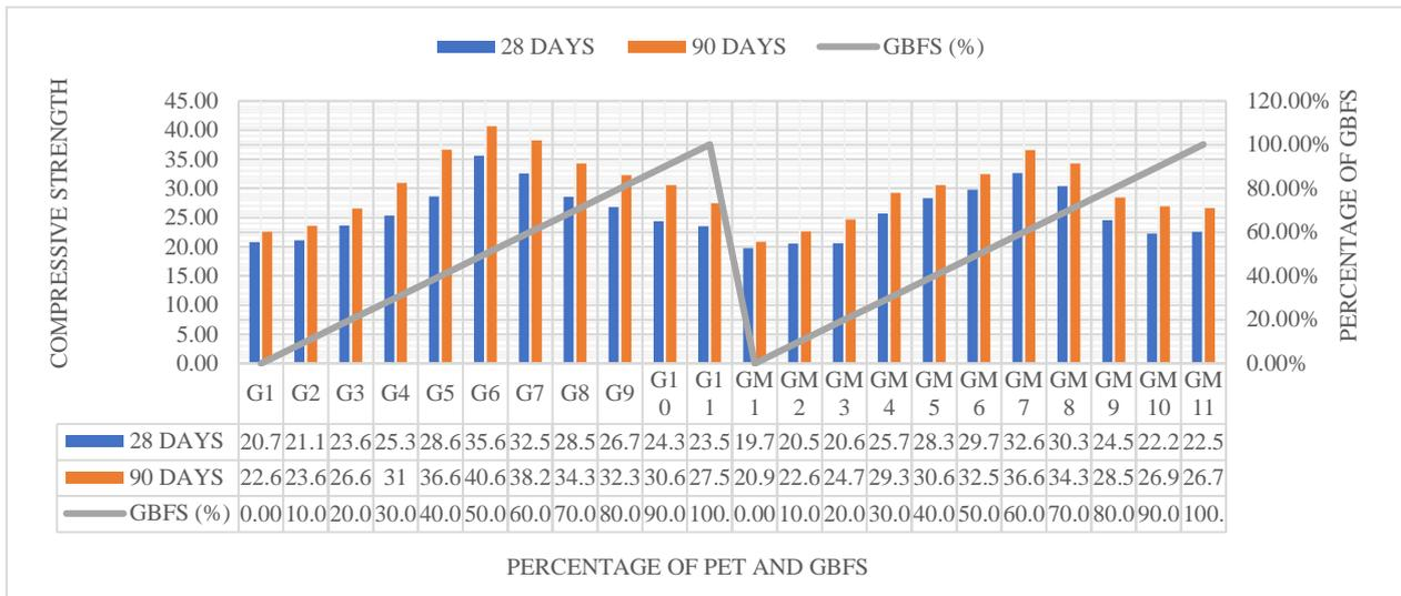
Fig. 8 - Compressive strength of samples with PET and GBFS [64]
