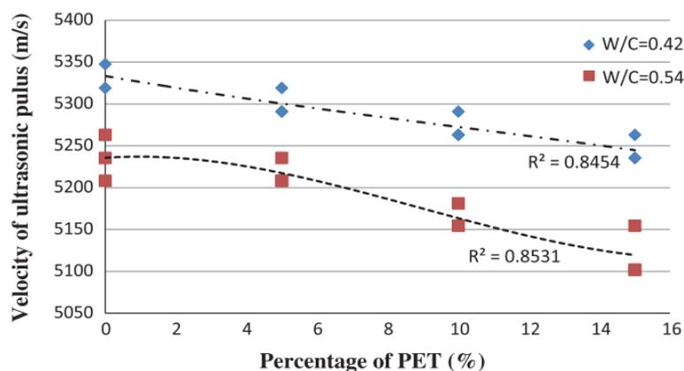
Fig. 3 - Result of Ultrasonic pulse velocity at 28 days with different water-cement ratios [50]
