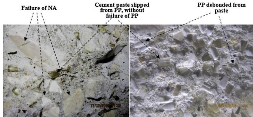
Fig. 2 - Photo of the concrete specimen after failure in the tensile splitting test [48]
