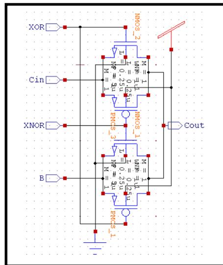
*Figure 4 Module III C<sub>OUT</sub> Circuit*
