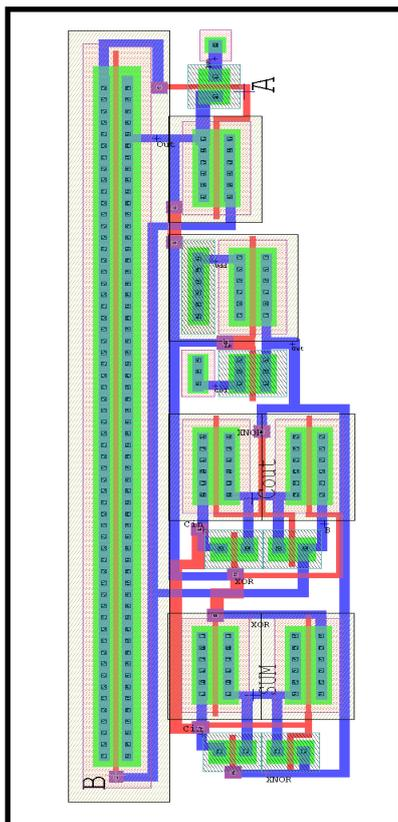
Figure 7 Layout for Hybrid Full Adder Circuit
