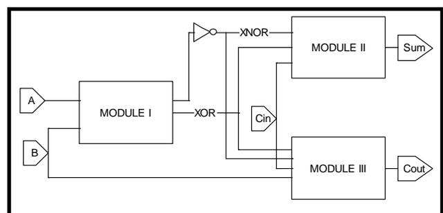
Figure 1 Block Diagram for Hybrid Full Adder
