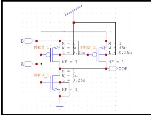
*Figure 2 Module I 3T XOR Circuit*
