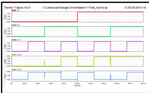
Figure 6 Output Waveform for Hybrid Full Adder Circuit
