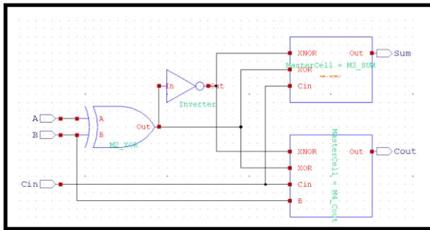
Figure 5 Schematic Diagram for Hybrid Full Adder Circuit
