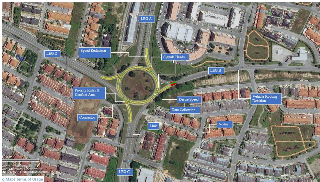
Fig. 9 - Two stop line signal roundabout network
