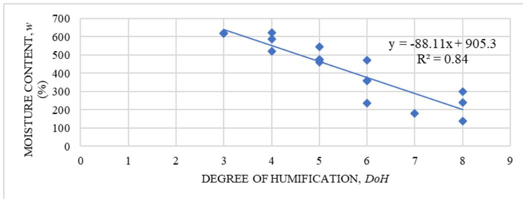
**Fig. 6 - Correlation between moisture content and degree of humification**
