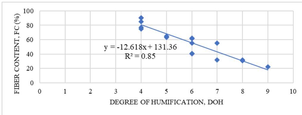
**Fig. 8 - Correlation between fibre content and degree of humification**
