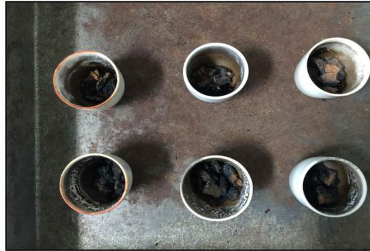
**Fig. 3 - Oven dried sample after being placed in muffle furnace**
