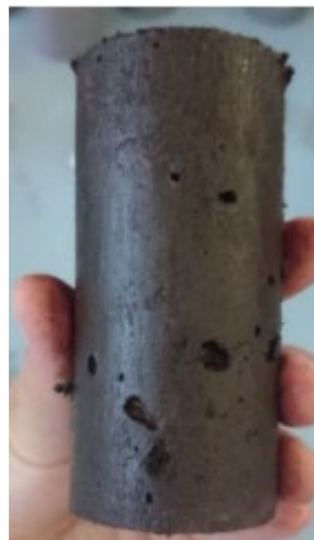
Fig. 7 - Voids present in the cement stabilized peat at 3.0 water additive ratio
