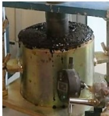
Fig. 10 - Condition of original peat during CBR after 28 days
