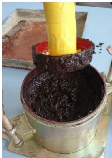
Fig. 4 - CBR peat sample compressed in 3 equal layers
