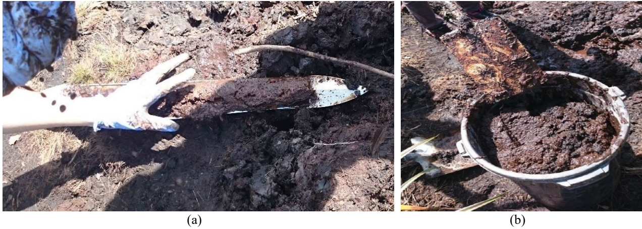
Fig. 2 – (a) Peat Auger sampling, and; (b) samples collected for further testing
