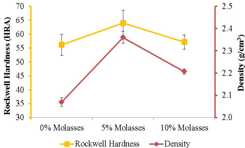
**Fig. 11** Relationship between density and rockwell hardness on crucible specimens
