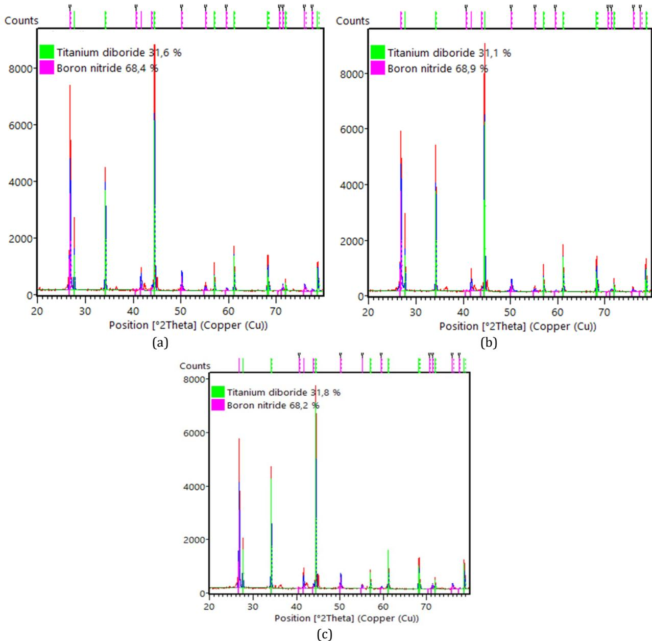
**Fig. 7** Rietveld analysis using high score plus software on the (a) 0% molasse; (b) 5% molasses; and (c) 10% molasses specimens
