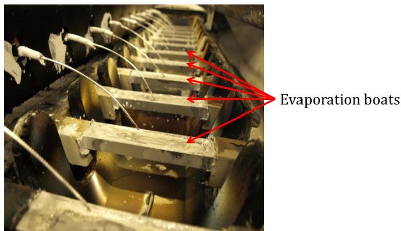
**Fig. 1** Evaporation boats in the plastic metallization process [6]
