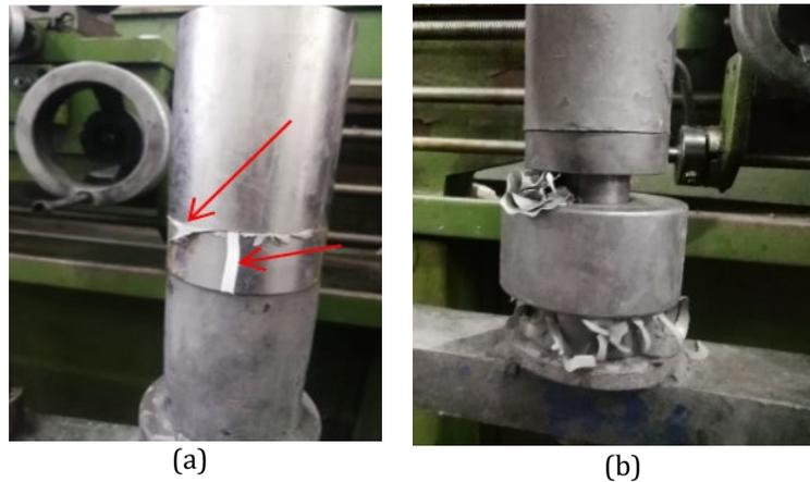
**Fig. 3** Green bodies that failed to form in (a) 15% molasses; and (b) 20% molasses specimens
