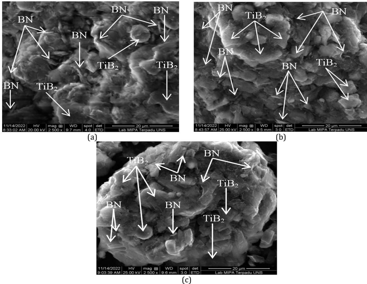
**Fig. 5** SEM images of the crucible specimens (a) 0% molasse; (b) 5% molasses; and (c) 10% molasses
