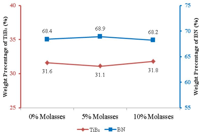
**Fig. 8** Comparison of weight percentage phase of BN and TiB<sub>2</sub> of the crucible specimens
