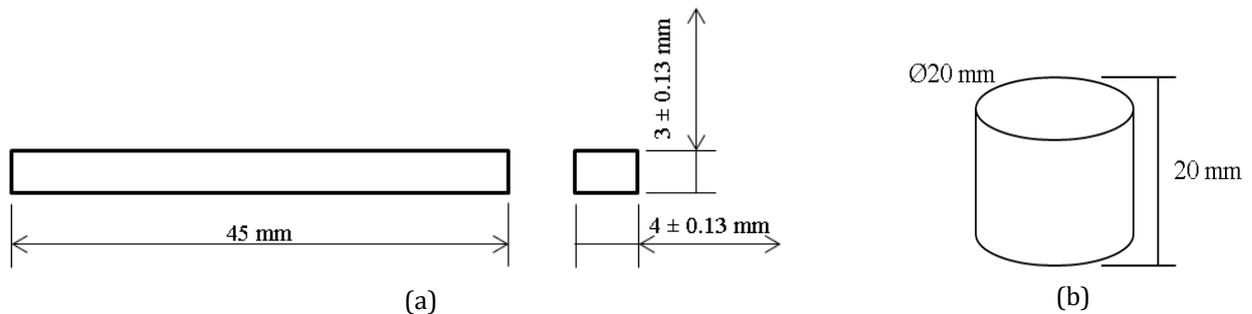
**Fig. 4** Specimen dimensions for (a) three-point bending; and (b) density testing
