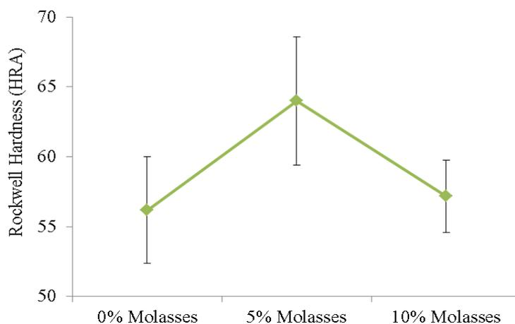
**Fig. 10** The effect of molasses concentration on the hardness produced in crucible specimens
