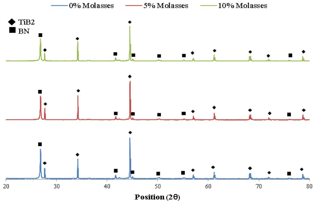
**Fig. 6** XRD pattern of the crucible specimens with various concentrations of molasses
