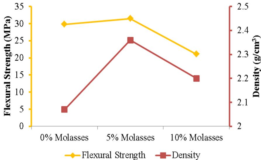
**Fig. 13** Relationship between flexural strength and density on crucible specimens
