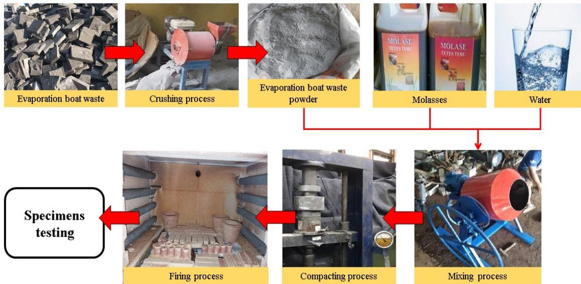
**Fig. 2** Schematic illustration of the process for fabricating crucible specimens
