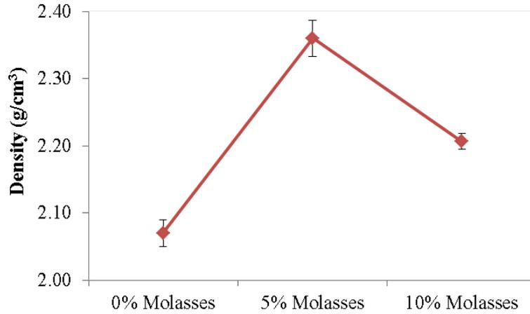
**Fig. 9** The density of the crucible specimens with various concentrations of molasses
