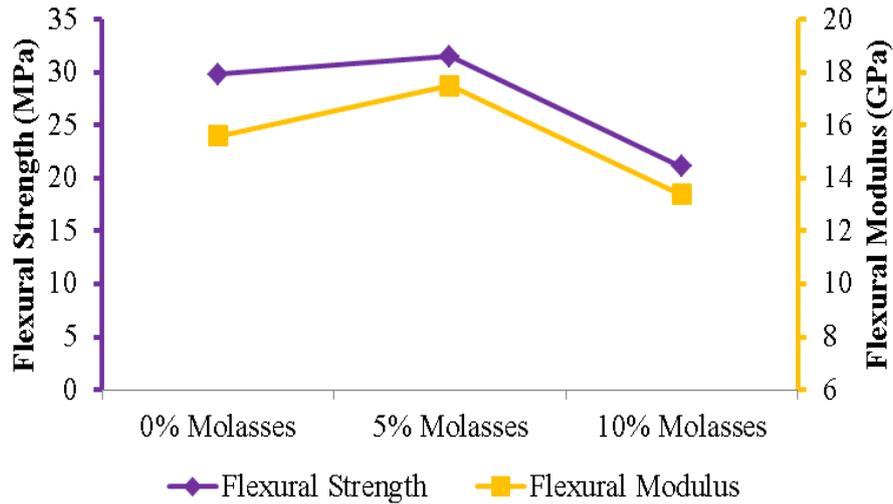
**Fig. 12** Flexural properties of the crucible specimens with various concentrations of molasses
