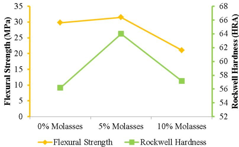
**Fig. 14** Relationship between flexural strength and rockwell hardness on crucible specimens
