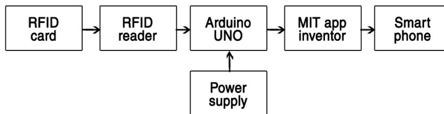
**Fig. 1 - Block diagram of the working time monitoring process**
