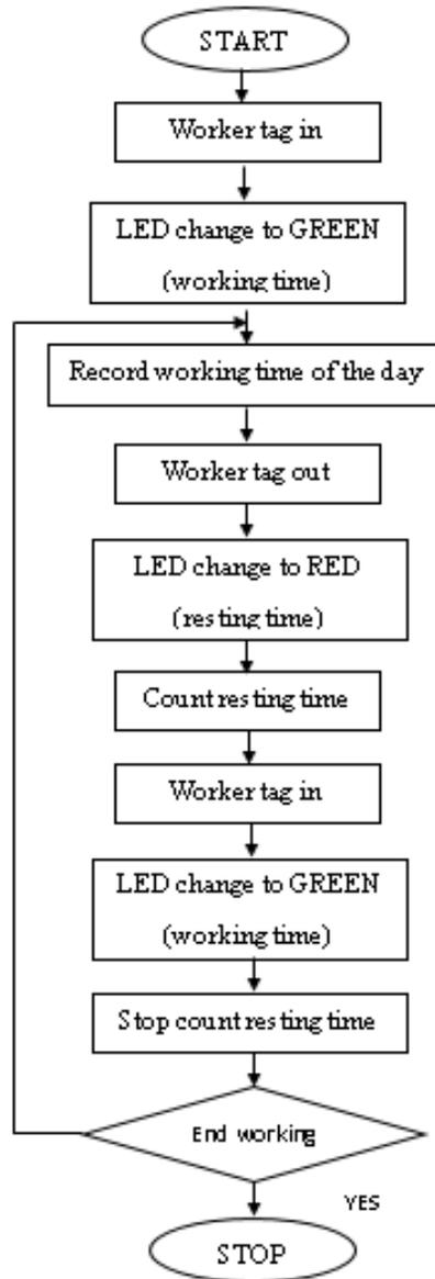
Fig. 2 - Flowchart of the monitoring system
