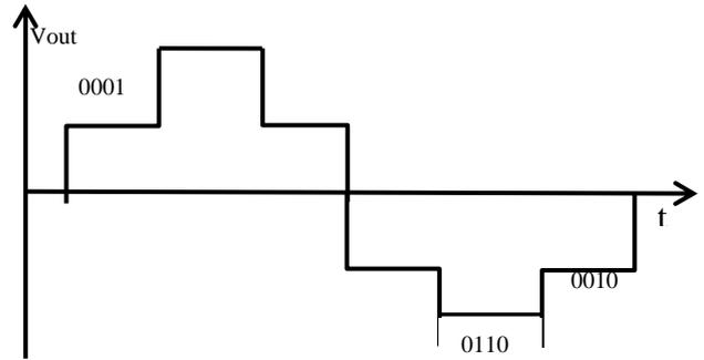
Fig. 2 Expected Result of Six Pulses Output Inverter Waveform.
