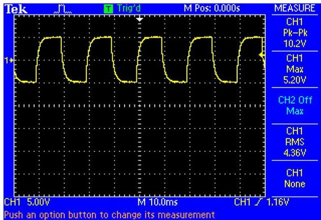
Fig.12 Inverter Output voltage.
