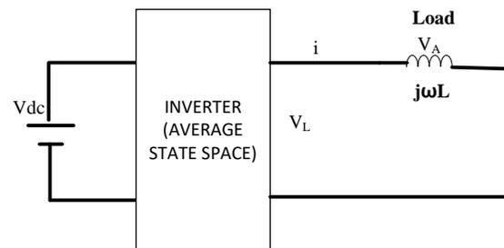
Fig.3 Average PWM Inverter Model.
