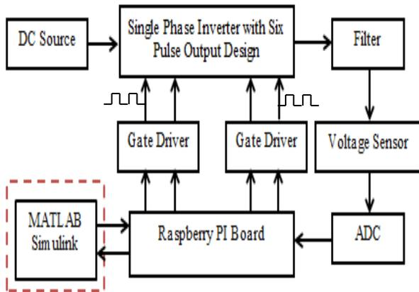
Fig.1 Block Diagram of the Project.
