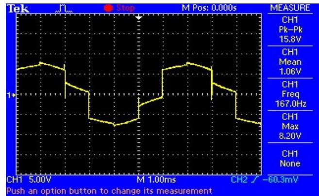
Fig. 6 Output Voltage Open Loop System.
