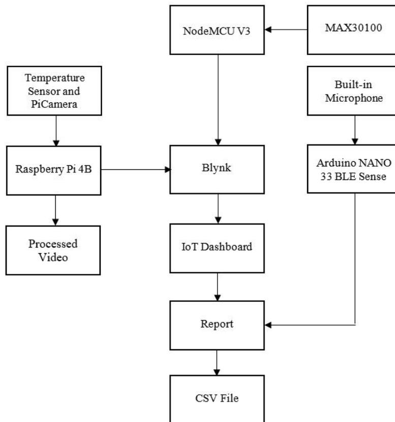
Fig. 1 System architecture of the IHDS
