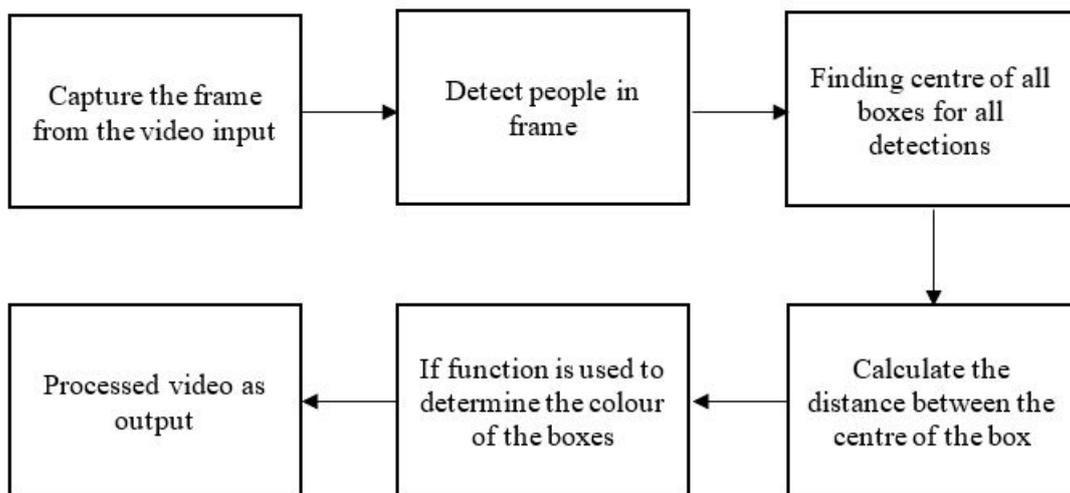
Fig. 2 The block diagram of the social distancing monitoring system
