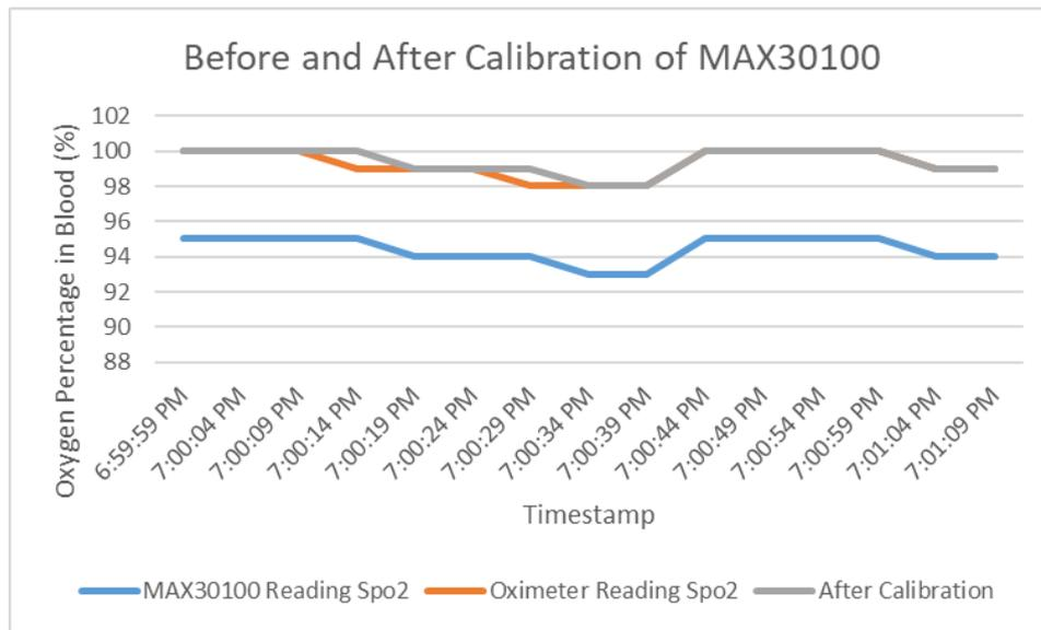
**Fig. 3** The SpO2 readings before and after calibration
