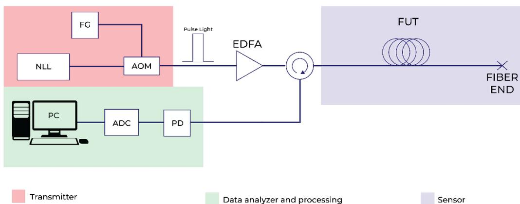
**Fig. 3**  $\Phi$ -OTDR based DAS system
