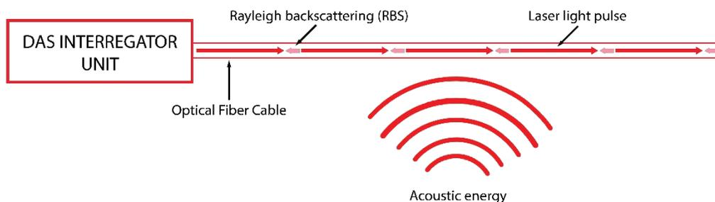
Fig. 1 DAS basic working principle
