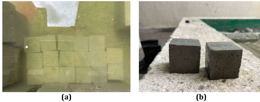
Fig. 1 Sample preparation (a) Curing process; (b) Mortar cube specimens
