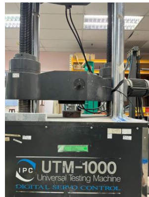
Fig. 3 1000kN Universal Testing Machine for compression test
