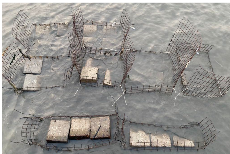
Fig. 1 Submerging the concrete sample in seawater at Kuala Perlis, Perlis
