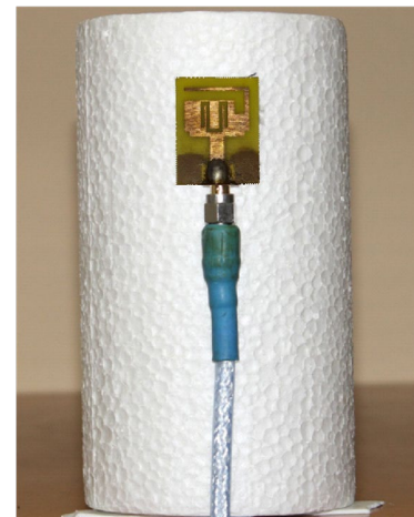
Fig. 3 UWB antennas' bent on styrofoam cylinder
