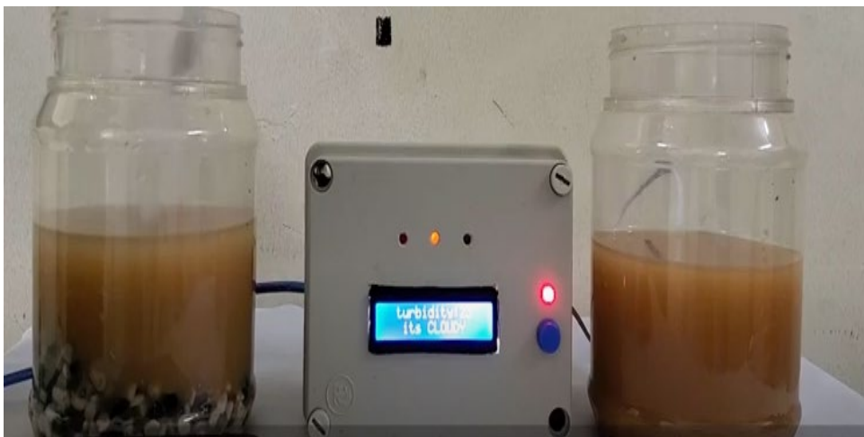
Fig. 8 Both bottles added potassium alum
