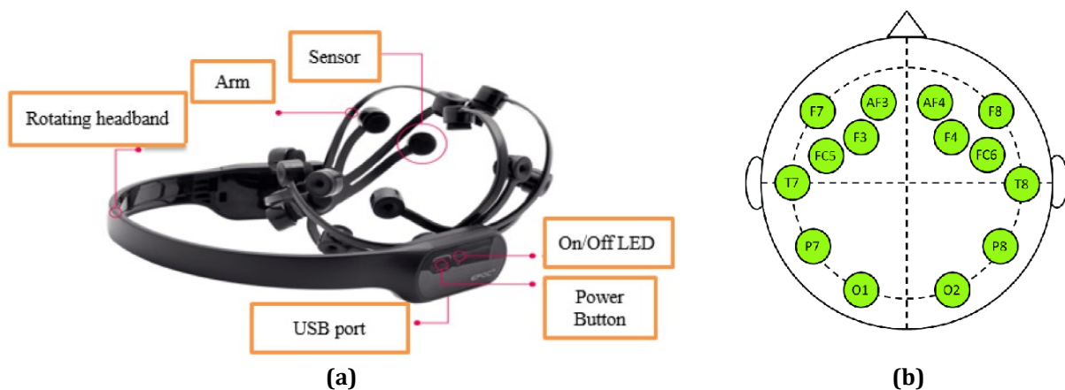
Fig. 2 (a) Emotive epoch X set and its function features; (b) The electrodes placement
