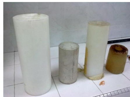
Figure 13: Left to right, Polypropylene log, concrete log, hollow polypropylene log, hollow wax log.
