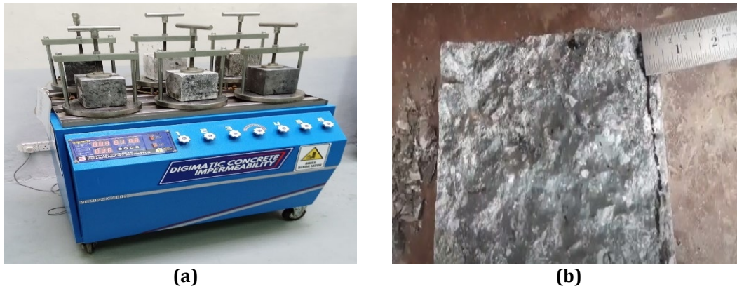
Fig. 4 Water permeability test
