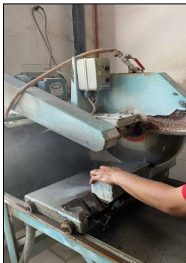
Fig. 2 The notch cutting process by using the saw cut
