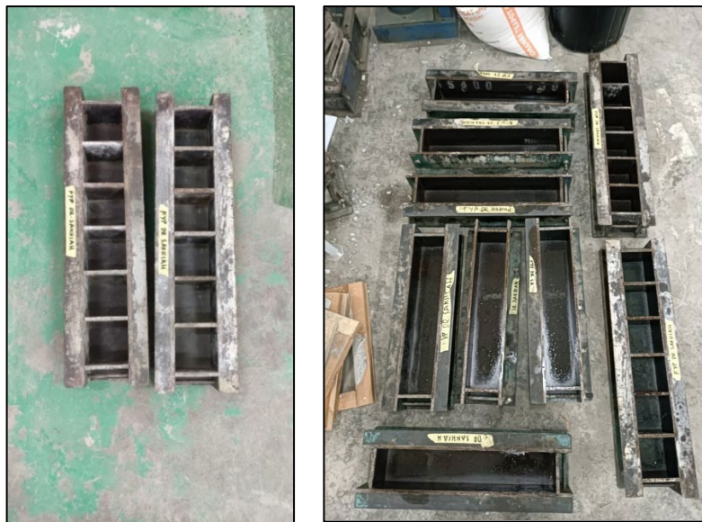
Fig. 1 Formworks that were used in the experiment consists of 12 cube formworks and oiled formworks
