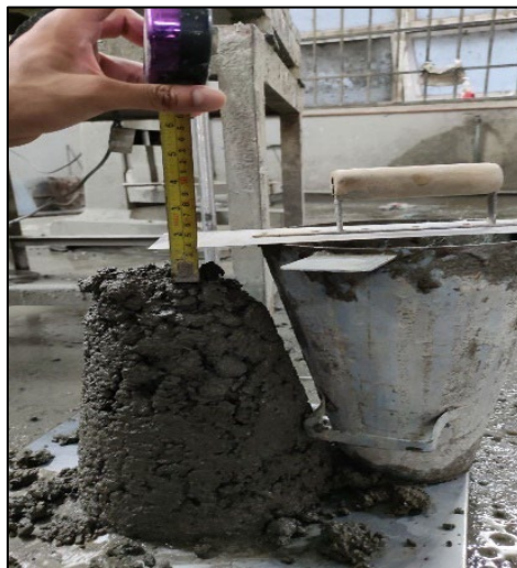
Fig. 4 The settlement of the concrete was measured by using measuring tape
