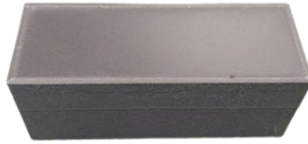
Fig. 4 Sample of 3D-printed PLA part before any post-processing
