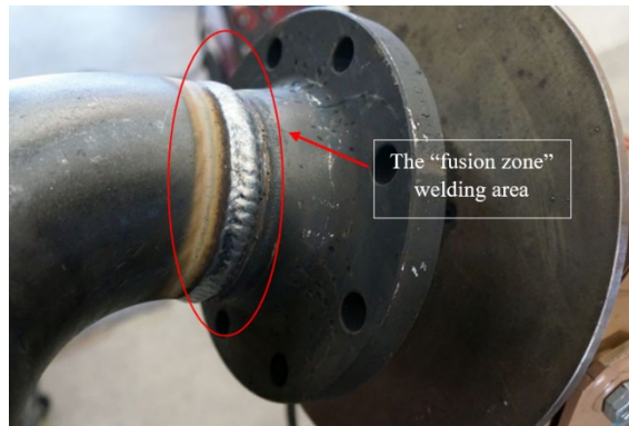
Fig. 4 Welding of CS pipe [33]
