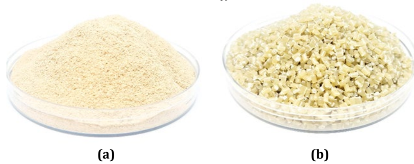
Fig. 1 The physical condition of material used in current research (a) 100 micron in size of RH; (b) RPP
