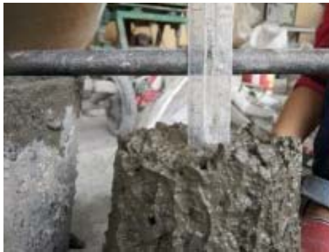
Fig 5: Slump test for each mix; (a) Normal Concrete, (b) 0.5% PET fiber, (c) 1.0% PET fiber, (d) 1.5% PET fiber, (e) 2.0% PET fiber
