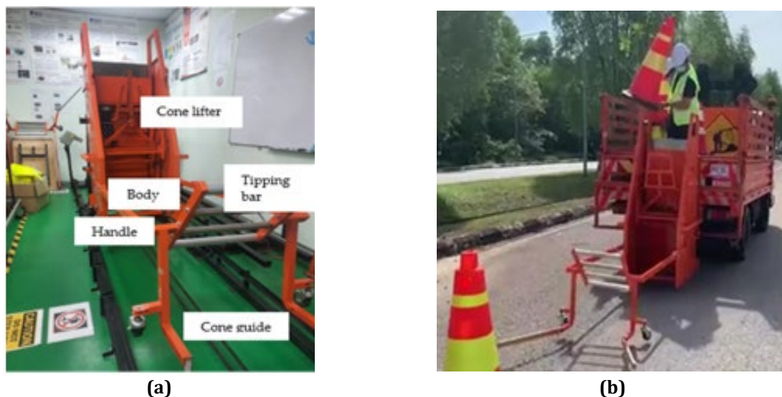
Fig. 1 Type of testing (a) Testing in the laboratory; (b) Testing in the field
