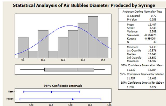
Fig. 5 Statistical analysis for diameter of air bubble produced by syringe at 20 ml volume[7]
