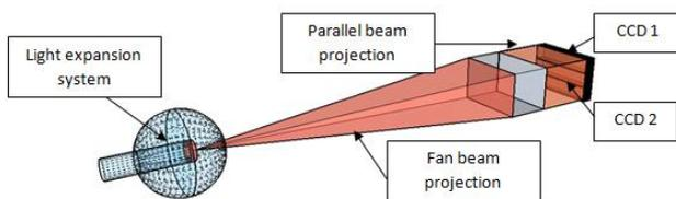
Fig. 1 Laser diode light expansion system
