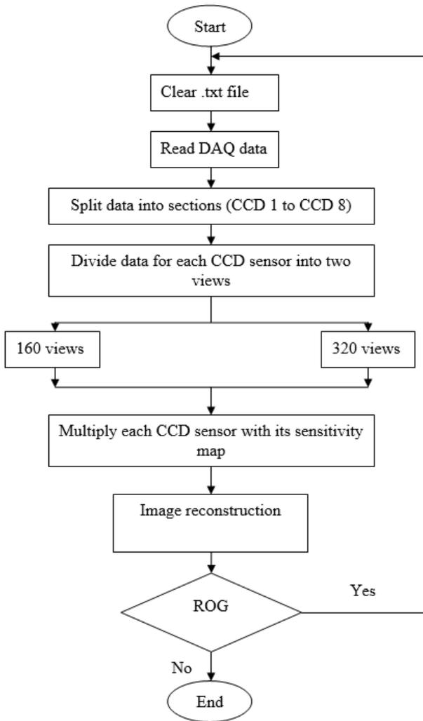
Fig. 4. Flow chart for reading real-time data for image reconstruction
