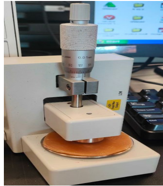
Fig. 2 The sample was placed between two electrodes on the dielectric test fixture
