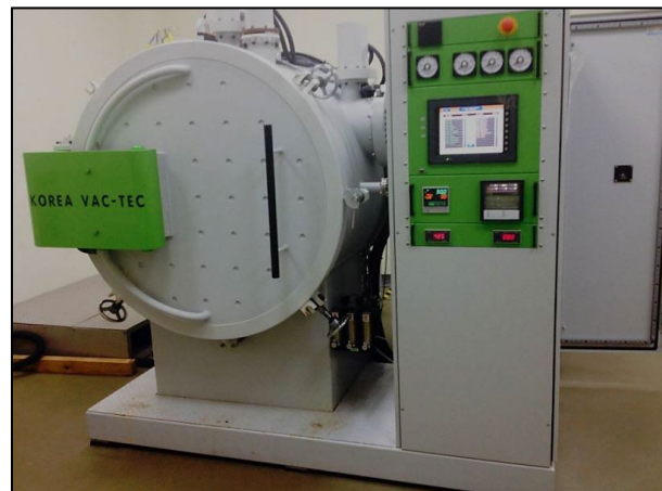
Fig. 3 KOREA VAC-TEC high temperature control atmosphere furnace
