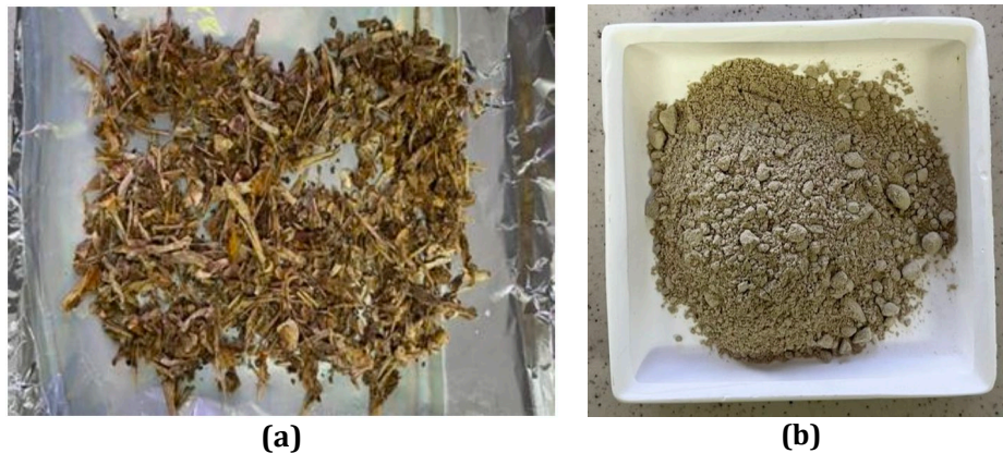
Fig. 2 (a) Dried chicken bone; and (b) dried chicken bone crushed into powder form
