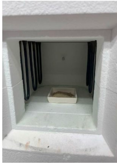
Fig. 3 Pulverized chicken powder is placed in the furnace for calcination
