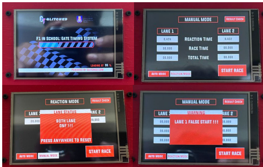
Fig. 11 Multiple display prompts on the Nextion display panel during operational of gate timing system
