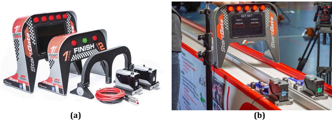
Fig. 1 (a) F1 in schools gate timing system; (b) Assembly gate timing system on the racetrack [6]
