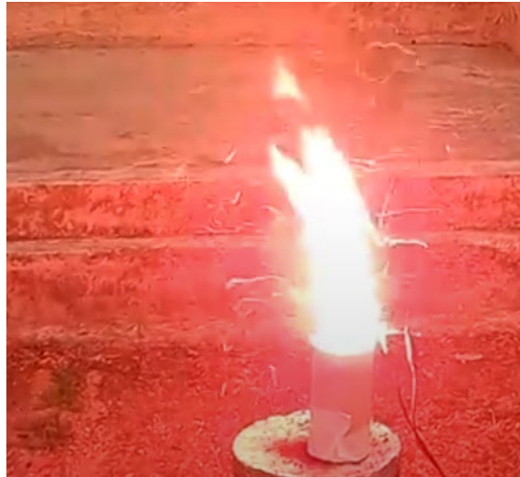
Fig. 4 FCA-4 testing at 30 seconds flare emission
