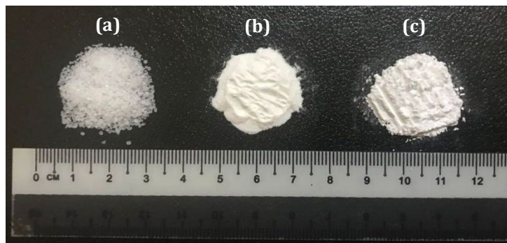
Fig. 1 Raw materials (a) PLA coarse powder; (b) PA12 powder; (c) WA powder
