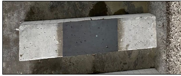
Fig. 2 Plain concrete beam with GFRP plate (100mm x 200mm) bonded to the surface using Sikadur-31 epoxy
