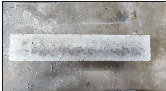
Fig. 1 Notch made by saw cutting under the beam
