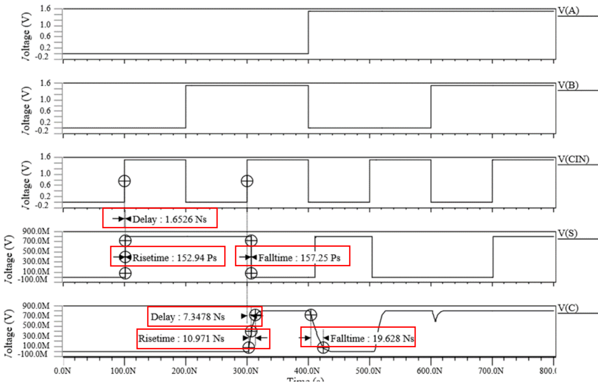
Fig. 23 The simulation waveforms of the 8 transistors full adder
