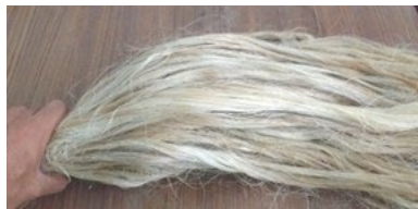
Fig. 2 Raw pineapple leaf fibre (PALF) before being cut to size as reinforcement
