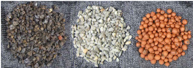
Fig. 3 Blackcinder (left), Pea Gravel (center) and right Clay balls (right) typically used in aquaponic system [9]
