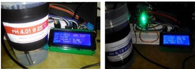
Fig. 8 Calibration pH sensor by using pH buffer powder
