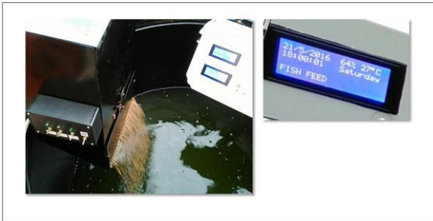
Fig. 21 Fish Feeder operation set by time
