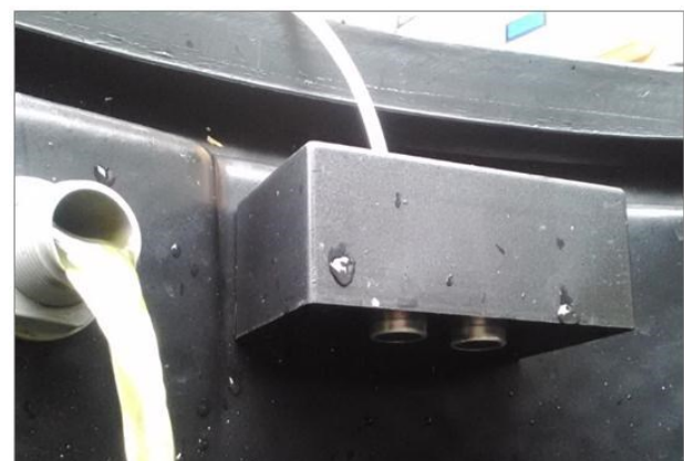
Fig. 20 The ultrasonic sensor used in this study
