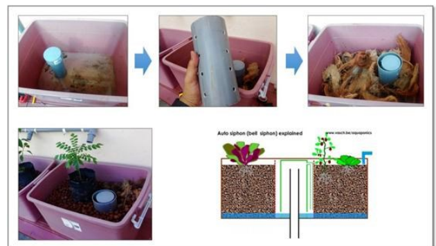
Fig. 11 Water filter using bell siphon concept.
